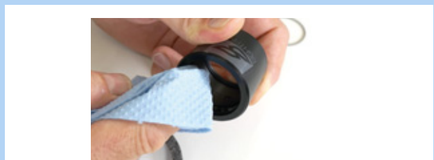
Figure 169: Cleaning the outer sleeve
