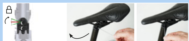
Figure 194: Closing the height adjustment
