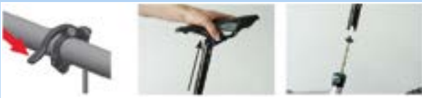
Figure 158: Pulling the seat post out
