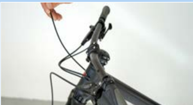
Figure 216: Attaching the end cap
