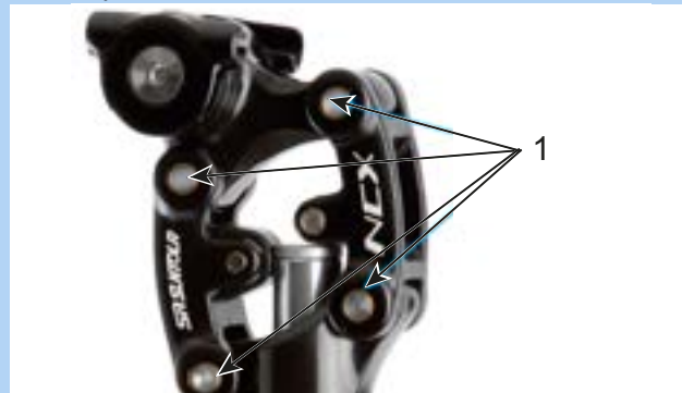
Figure 156: SR Suntour suspension seat post lubrication points
