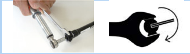
Figure 179: Setting in a clockwise direction
