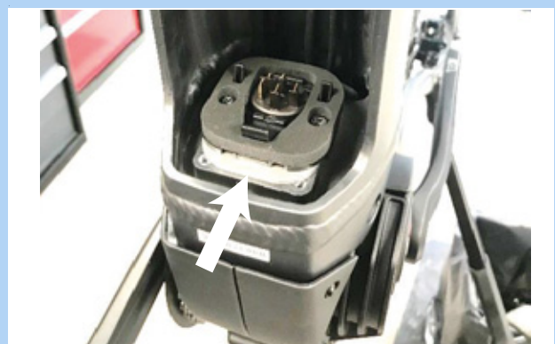
Figure 54: Fitted adapter plates
