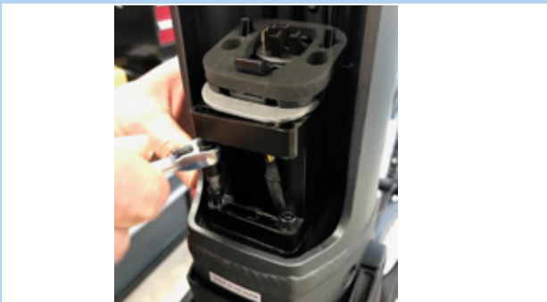
Figure 51: Removing the 4 mm hexagon screws
