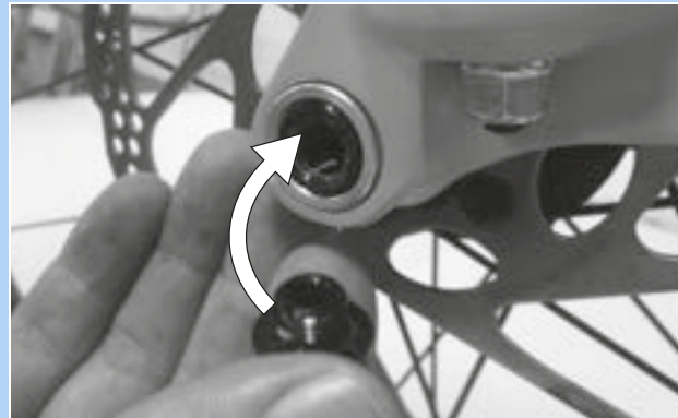
Figure 67: Pushing the quick release lever into the axle
