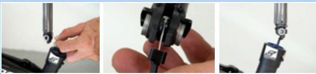
Figure 215: Attaching and pushing in the seat post
