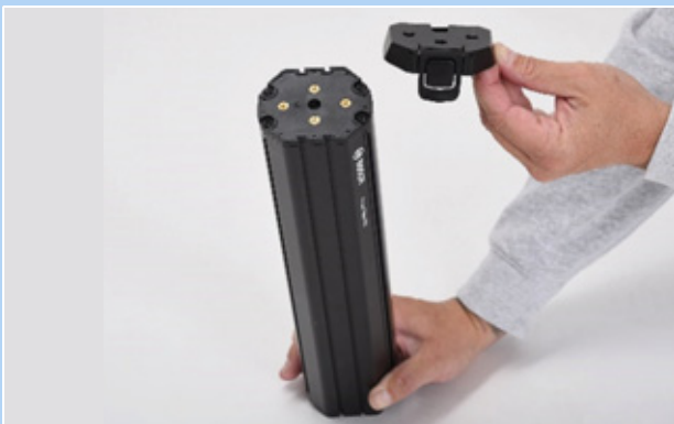
Figure 57: Fitting the mounting plate
