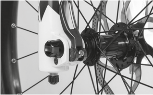
Figure 73: Perfect position for the clamping lever
