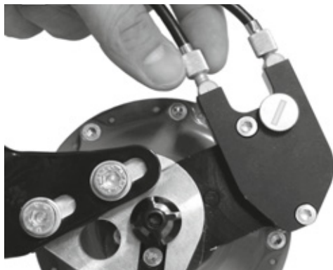
Figure 150: The tension adjuster on Rohloff hub versions with external switch control is located on the cable box positioned on the left-hand side
