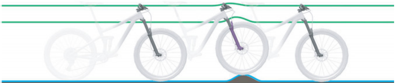
Figure 10: Optimum fork riding performance over bumps
