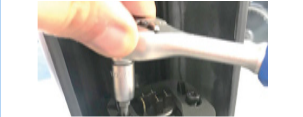
Figure 50: Undoing screws on battery mount
