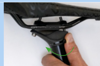
Figure 213: Closing the height adjustment
