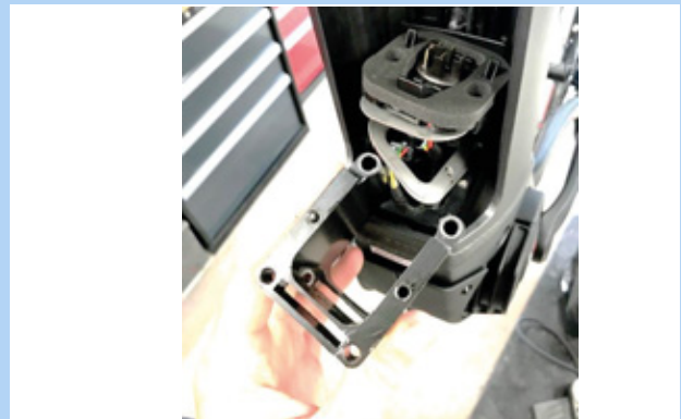
Figure 53: Pulling out the PowerTube adapter
