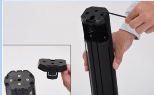
Figure 61: Fastening the battery mounting plate
