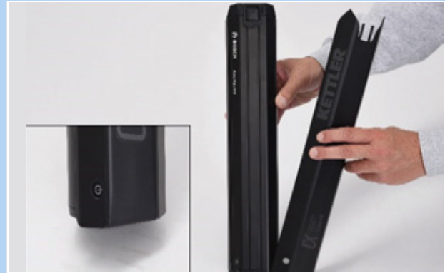
Figure 58: Pushing the battery cover onto battery
