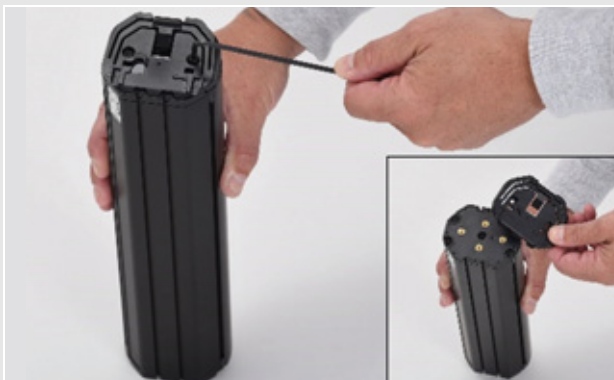
Figure 32: Detaching the upper interface
