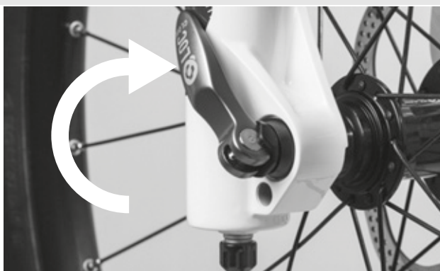
Figure 54: Closing the quick release
