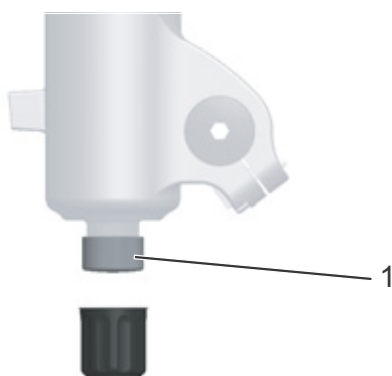
Figure 73: FOX rebound adjuster (1) on the fork end
