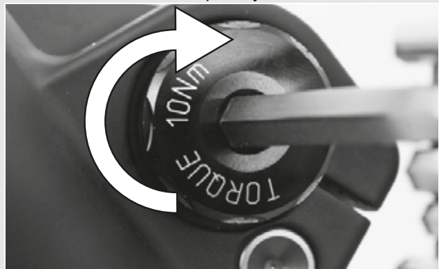
Figure 43: Tightening the inserted axle
