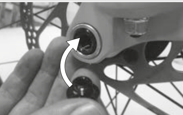
Figure 41: Pushing the quick release lever into the axle
