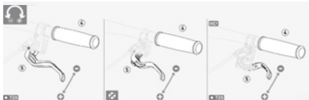
Figure 68: Setting the grip distance on a Magura disc brake lever
