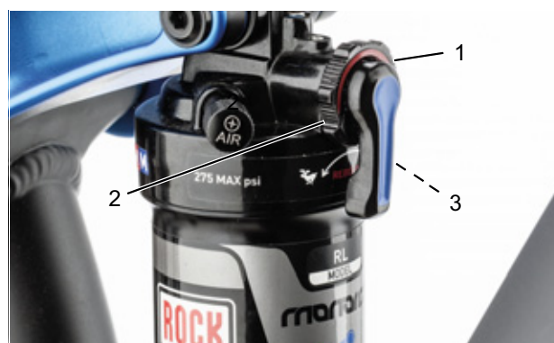
Figure 88: Setting the rebound damper strength on the rear frame damper setting wheel (1)
