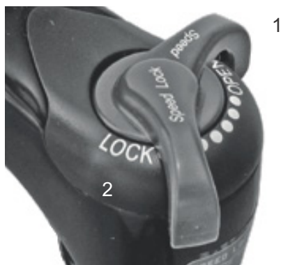
Figure 87: Suntour compression adjuster with OPEN (1) and LOCK (2) positions
