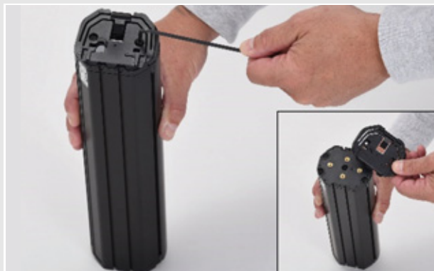
Figure 35: Detaching the upper interface
