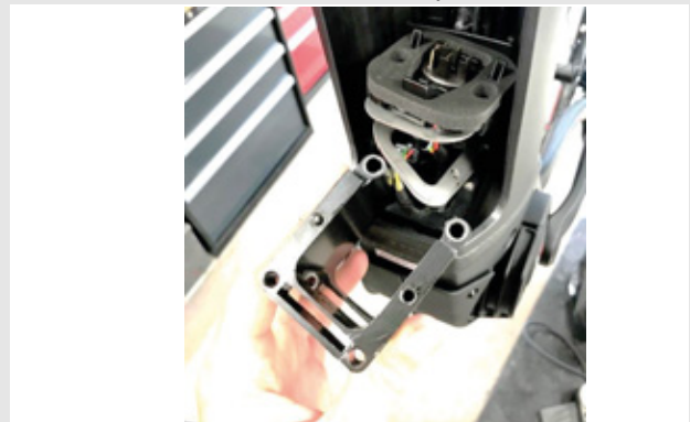
Figure 29: Pulling out the PowerTube adapter
