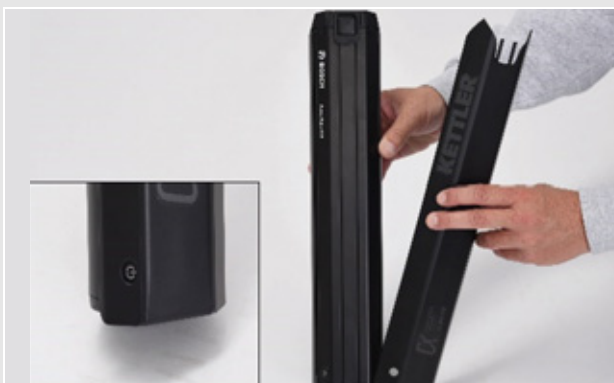
Figure 34: Pushing the battery cover onto battery
