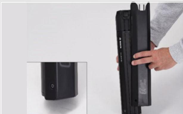
Figure 38: Pushing the battery cover onto battery
